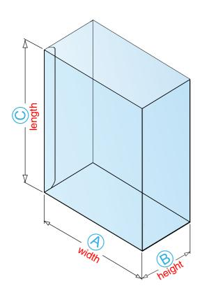
A Sleeve is used in combination with another packaging component. It's frequently used as a slip-on cover for a paperboard carton or tray, or an open set box structure. Sleeves can also be used in combination with injection molded or vacuum-formed plastic end caps or inserts.
