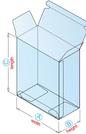
Straight Tuck cartons have both top and bottom panels that hinge off the carton's front panel. The top and bottom panels fold from the front and tuck to the rear, providing a clean front panel appearance. This style carton is appropriate for both hand and machine forming and filling applications.
