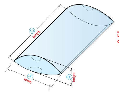
Pillow Packs are a cost-effective style of packaging, typically used for products of shallow depth or for bulk packs of small items. A wide variety of features can be included to provide added utility, i.e.: thumb locks, standing bottoms, or hang tabs.
