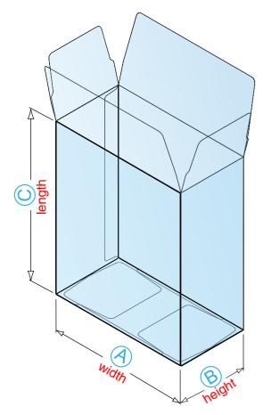
The Seal End carton is typically erected, filled and sealed on automated packaging equipment. Since the top and bottoms are glued closed, it offers tamper evidence as compared to tuck style cartons.
