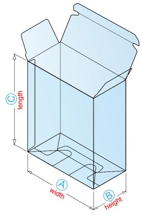
123-Bottom cartons are designed for efficient hand set-up and loading. Although not as efficient as Auto-Bottom cartons, this carton style is also used when faster set-up is desired but production volume or the package's contents are not suitable for automatic packaging equipment.
